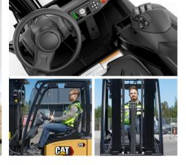
The adjustable seat and steering column assure a perfect driving position for drivers of all sizes. Forward, downward and side views are excellent due to a specially designed free lift cylinder structure where hoses and chains are positioned to minimise obstacles to vision. Ergonomic controls include an adjustable armrest, with inbuilt fingertip levers, and a set of low-fatigue pedals.
